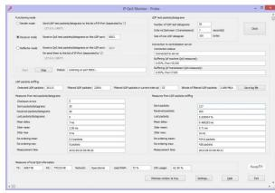
In Sender mode, the probe can **simulate UDP traffic** by sending test packets to a probe working in Receiver mode.
